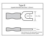
Although the above diagram show the spades being flat, we reccomeng using spade connectors that have a 30-45' bend. This allows the speaker wire to exit the amplifier at an angle rather than straight down.
